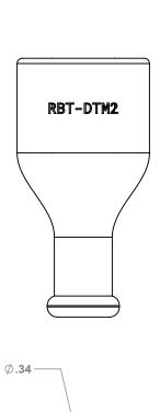
IF ADDITIONAL TAIL SEALING IS REQUIRED, A SHORT PIECE OF APPROPRIATELY SIZED ADHESIVE-LINED HEATSHRINK TUBING CAN BE USED.
